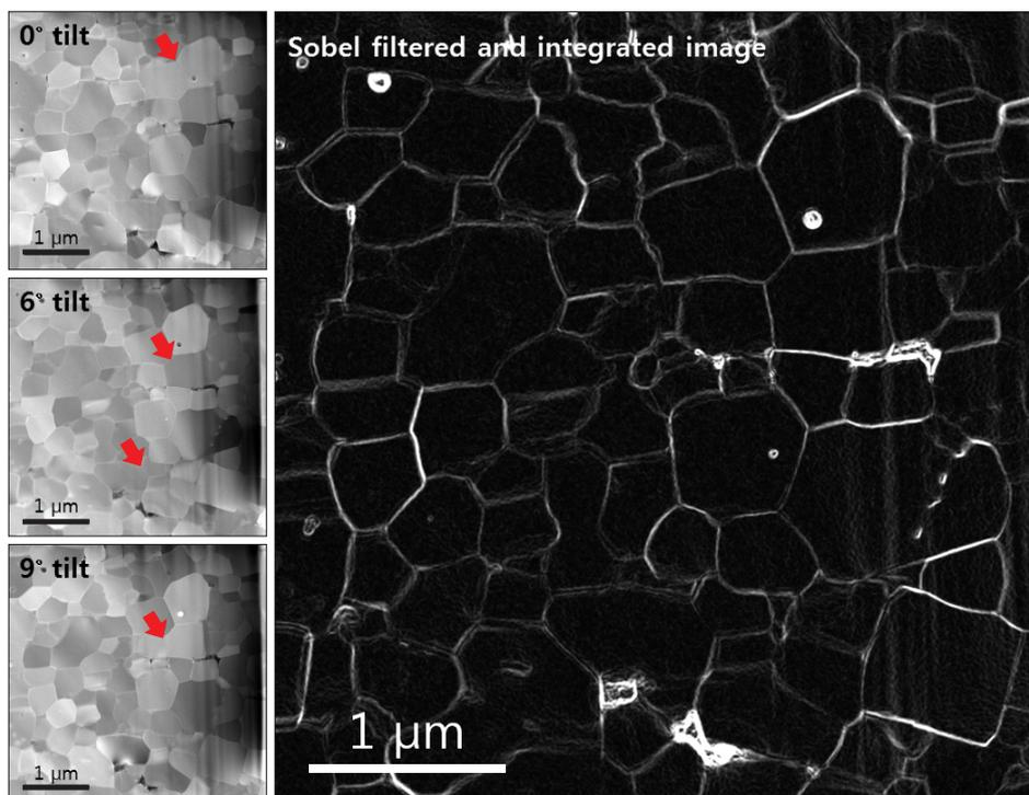
Generally, the grain size has a great influence on the physical properties of a material (Pauli et al., 2014). To accurately measure the grain size from the conventional images, computer process so called Sobel filter (Sobel et al., 1968) can be used. It computes gradient change between neighboring pixels and emphasizes the outline of objects.
