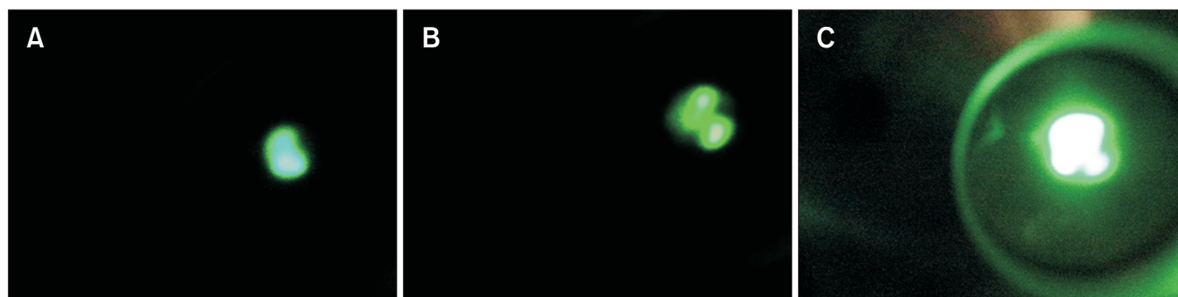
Fig. 1.2. Images of field emission from clean tungsten tip are distributed in several spots, when increasing the voltage. The emission current was getting brighter. As can be seen from the emission images, emission spots start to become brighter or bigger as the voltage was increased. Image details are: (A) 780 V, 51 nA; (B) 870 V, 100 nA; (C) 960 V, 5.50 nA.
